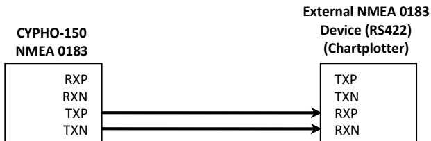
Figure 8 NMEA 0183 Connection illustration
