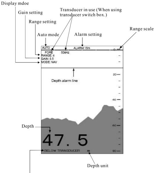
Explanation of depth (Below transducer, or below surface)
