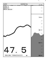
If the range scale for both the Contour and Strata display must be the same. If they are not, the message "OUT OF RANGE" appears. The update of the contour data may take max. one minute. Wait for one minute to display accurate contour if you change the range scale.
