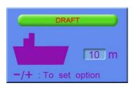
3. Press the [+] key to increase the setting depth and [-] key to decrease it. The setting depth is -10 to 30 m in steps of 0.1 m.
