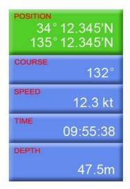
There are two kinds of OS DATA displays: DATA 1 and DATA 2, as selected on the system menu. DATA 1 is the default setting, and it is shown in the figure above. The DATA 2 display is as below.
