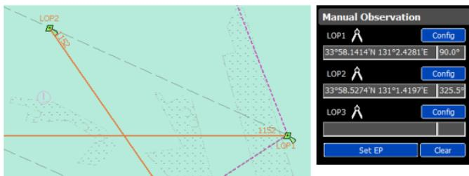
**Set EP:** it is calculated via the system, to predict whether there was a position of the ship. The prediction is display on the chart with a timestamp. As shown in figure below:
