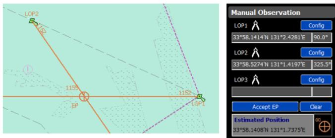
**Estimated Position:** display EP coordinates and it also provides Position Fix as a Marker Symbol.
