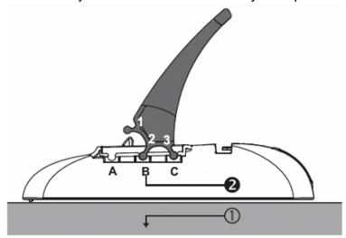
Step 2: Place with two hands on the stand of the EDM and firmly press down the stand, the "2<sup>nd</sup>" antler will be pulled straight out of the slot "B" hole; Keep pressing down the stand, the "3<sup>rd</sup>" antler will be pulled straight out of the slot "C" hole.
