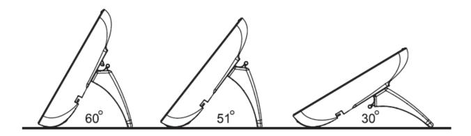
After unpacking the box, install the stand on the EDM first. Here we illustrate an example below of 60° angle installation with the stand. There are three sets of "antlers" on the top of the stand (named 1, 2 and 3) and there are three sets of mounting slots on the back of the EDM (named A, B and C). See the illustration below.
