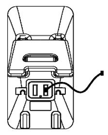
**Step4:** Plug the other end of the SATA cable into the SATA connector of the phone.
